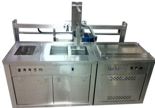
■ Gantry Automatic Cleaning System
