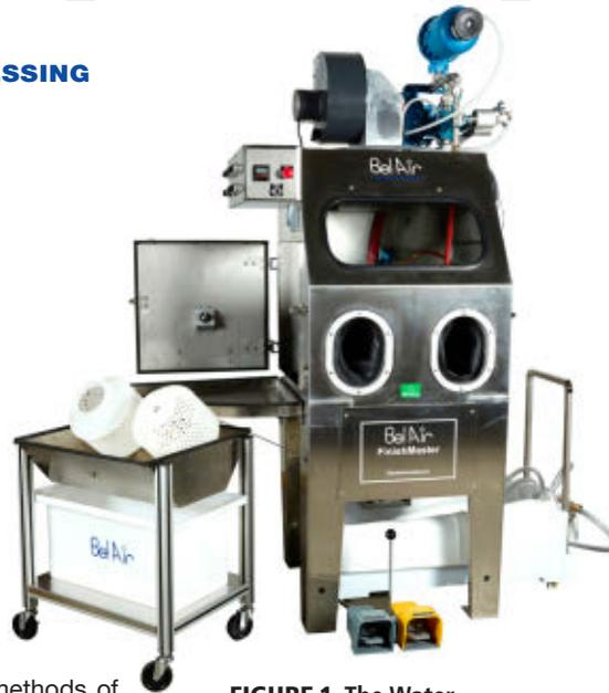
**FIGURE 1.** The Water Jet Slurry Blaster is one of the best ways to remove powdered build material from parts.
