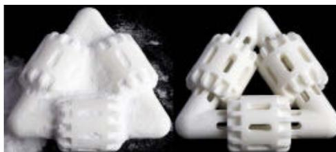
**FIGURE 2.** This plastic part was printed and Water Jet Slurry Blasted to remove build material.
